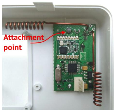
Figure 16. "Ajax uartBridge" radio receiver in the CP housing
