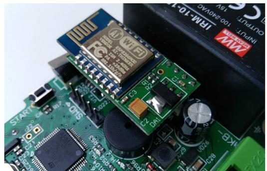
Figure 18. Installation of WiFi module
