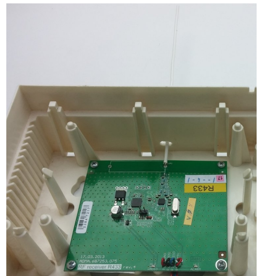
Figure 21. “R433” rev. 4 radio receiver in the device housing
