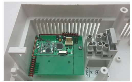
Figure 31. Ajax "uartBridge" radio receiver in the device housing
