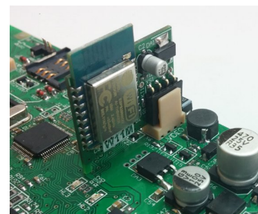
Figure 38. Installing «W11M» to X6 connector
