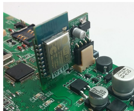
Figure 38. Installing «W11M» to X6 connector
