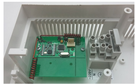
Figure 31. Ajax "uartBridge" radio receiver in the device housing
