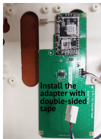
Figure 29. Adapter «L25_Crow_rev3» in the device housing
